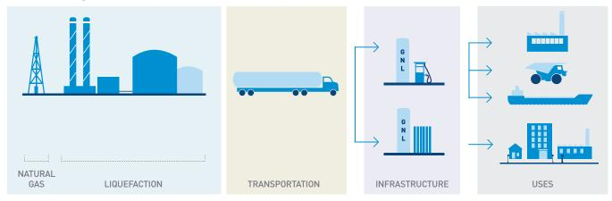
By liquefying natural gas, which takes up 600 times less volume than in its gaseous state, it can be stored and transported reliably, safely, and economically.
