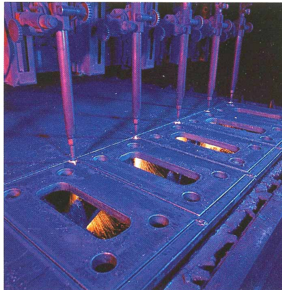
OXYFUEL GAS CUTTING USING NATURAL GAS AT DRUMMOND McCALL
